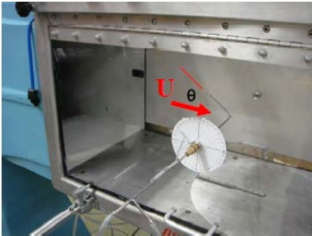
FIGURE C-1 Experimental Test Set Up (left) to Determine the Dependence of the Angle of Attack on the Coefficient of Pressure (right).
